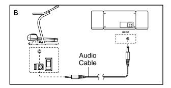
C. Plug one end of the audio cable into the jack on the side of the hiker near the power cord. Plug the other end of the cable into a 3.5mm Y-adapter (available at electronics stores). Plug the Y-adapter into the PHONES jack on your stereo. Plug your headphones into the other side of the Y-adapter.
